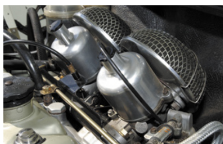
Most visible signs are twin 1½” carbs with single-piece heatshield, Ram-Flo air filters, and handbrake warning light.
