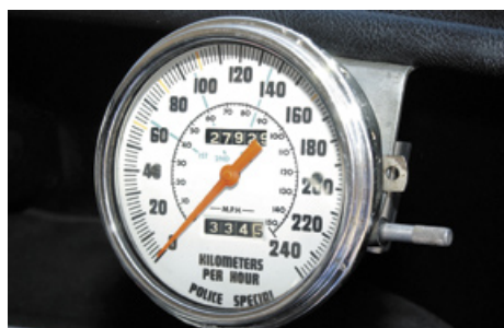
NSW pursuit cars had special speedos. This one, being km/h and mph is c1973-75.
