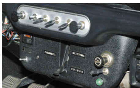
Unusual heater cover - Italian labels.
