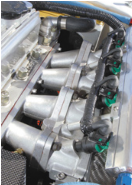
Elder crossflow head and DC&O injection.
