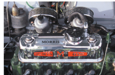
Sports 850 twin-carb setup. Note layout of float chambers
